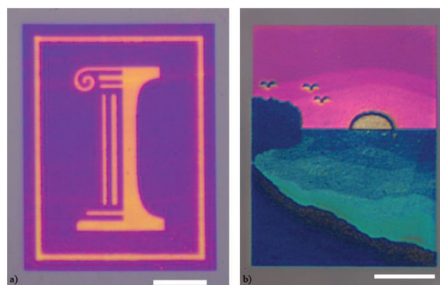
Figure 4. Microscope optical images on \text{AgIAgPO}_3 produced by patterned electron beam irradiation. a) Optical image of high-contrast bicolor graphic. Patterned in two passes: 5 and 7 \text{ kV } V_{\text{acc}} . b) Optical image of gradient painting pattern in two passes: 4 and 6 \text{ kV } V_{\text{acc}} . Scale bars are 25 \text{ }\mu\text{m} .
